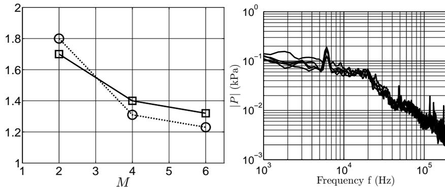
**Fig. 7** Left: Amplification factor for the six computed cases circle,  $\gamma = 1.4$  square symbol,  $\gamma = 1.2$ . Right: Spectra from measured pitot noise in the Caltech Ludwig Tube at  $M = 4$ .
