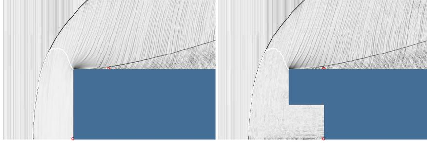
**Fig. 2** Pseudo-schlieren images of flow over pitot tube. The greyscale is a monotonic function of the fractional density gradient. The white line is the sonic line.  $M = 4$ ,  $\gamma = 1.4$ . Left: Without cavity, Right: With cavity
